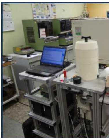
Figures 3 and 4: Testing of the CIEMAT and PTB Ge-based prototype spectrometric devices at end-user facilities in Portugal (Siderurgia Nacional) and Czech Republic (Vitkovice Steel)
