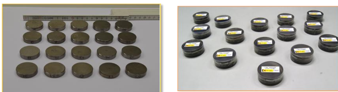
Figures 1 and 2 (above): Two sets of reference standards; one set from slag contaminated with Ra-226 and one set from cast steel contaminated with Co-60 (respectively)
